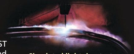
Simulated lightning test with no product failure
